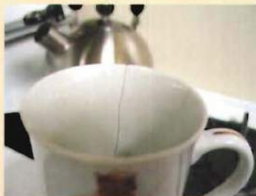
The coffee mug cracked after boiling water was poured into it.
