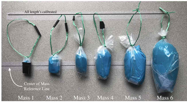
Figure 1. Size comparison of the masses used to measure the oscillations of the homemade pendulum. The mass on the left is approximately 5-10g while the mass on the right is in excess of 150g.
