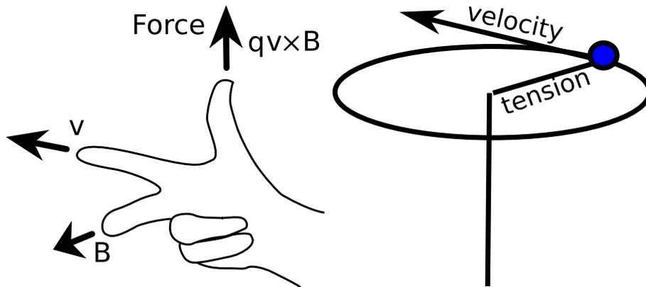
Figure 1: Finding the direction of the force ( $F$ ) from a magnetic field ( $B$ ) on a charge with velocity  $v$ . When an object moving at constant velocity experiences constant acceleration that is perpendicular to the velocity, it moves in a circle.
