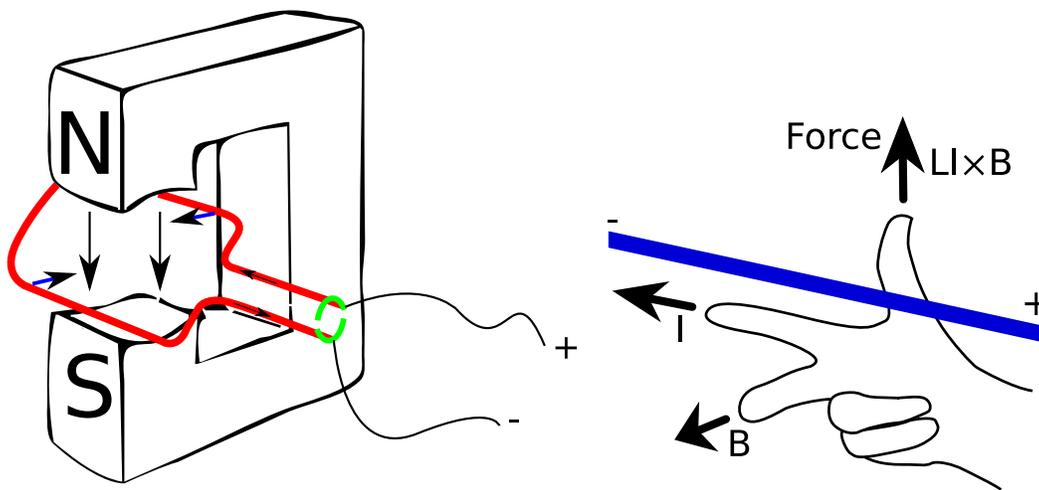
Figure 2: A simple motor described in this lecture. The right hand rule tells us that the force on a length of wire (direction of thumb) is perpendicular to the direction of the current flow and the magnetic field. The net force drives the loop counter-clockwise.
