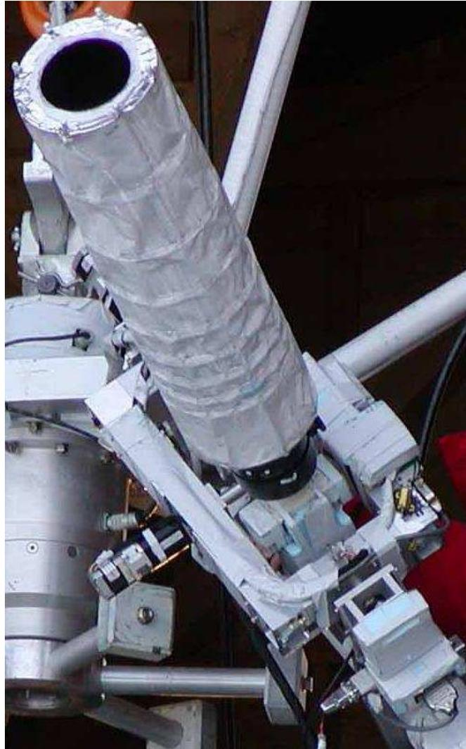
Figure 3.12: Flight ready star camera. The stepper motor drivers and encoders are covered in foam in an effort to prevent freezing at float altitude.
